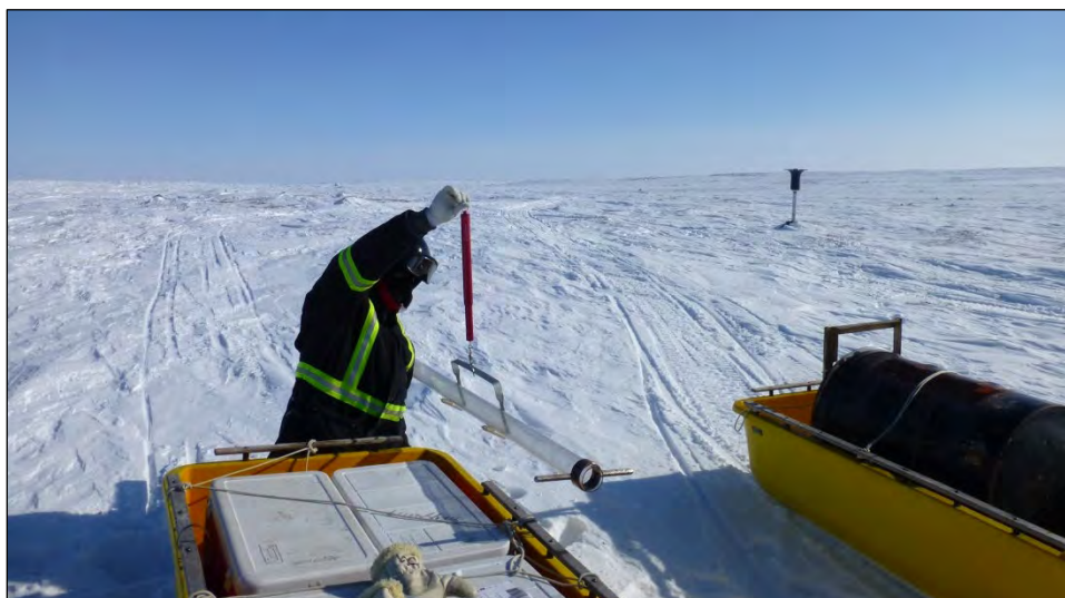
Photo 2.2-1: Snow core sample being weighed, with dustfall gauge in background.
