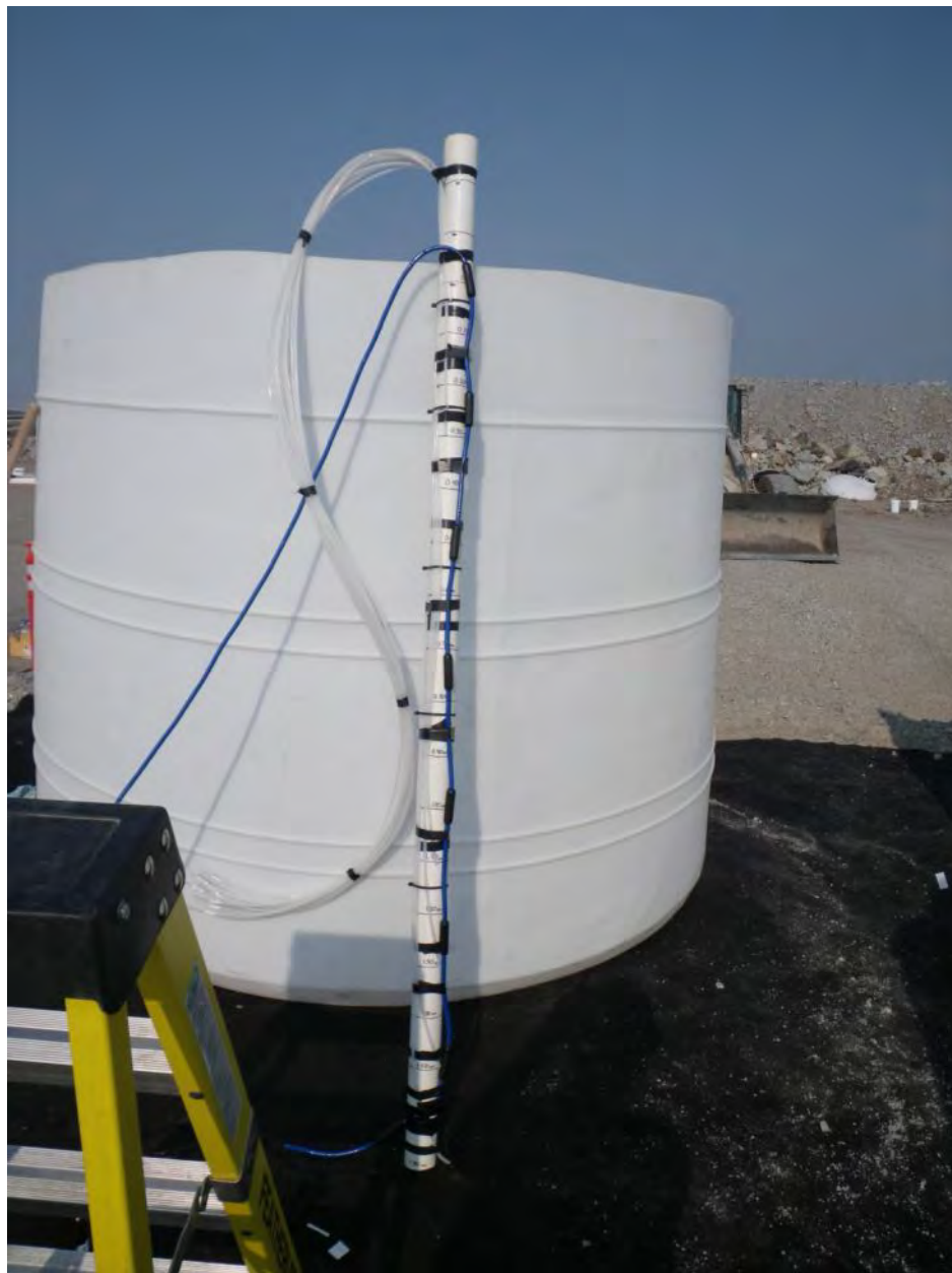
Fig. 3. Central pipe with gas lines and thermistors attached.
