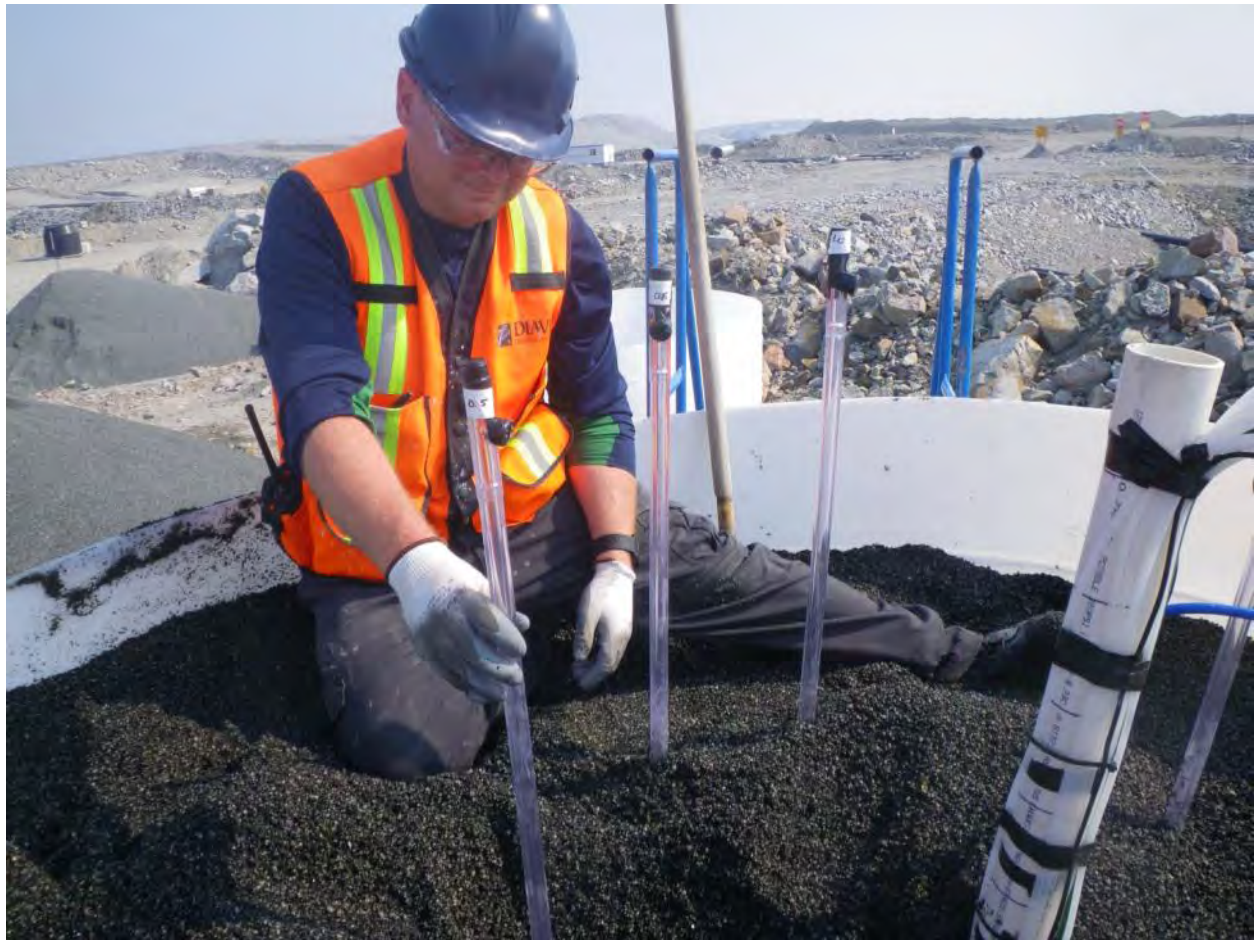
Fig 5. Installing 0.25 m tensiometer in filled CPK tank.
