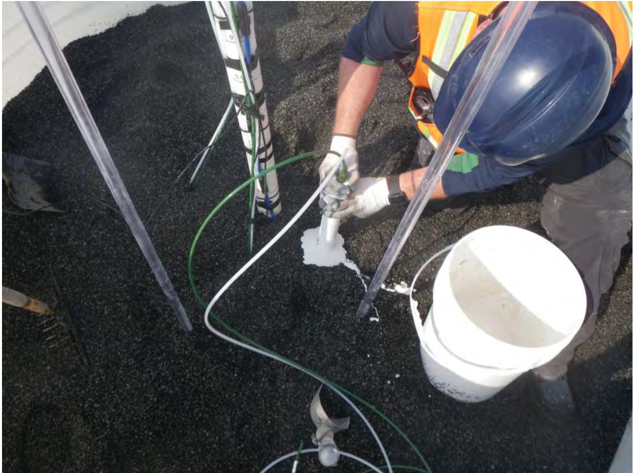
Fig. 4. Installing SWSS. Silica flour slurry was placed around porous ceramic cup to establish good contact between the ceramic cup and the CPK.
