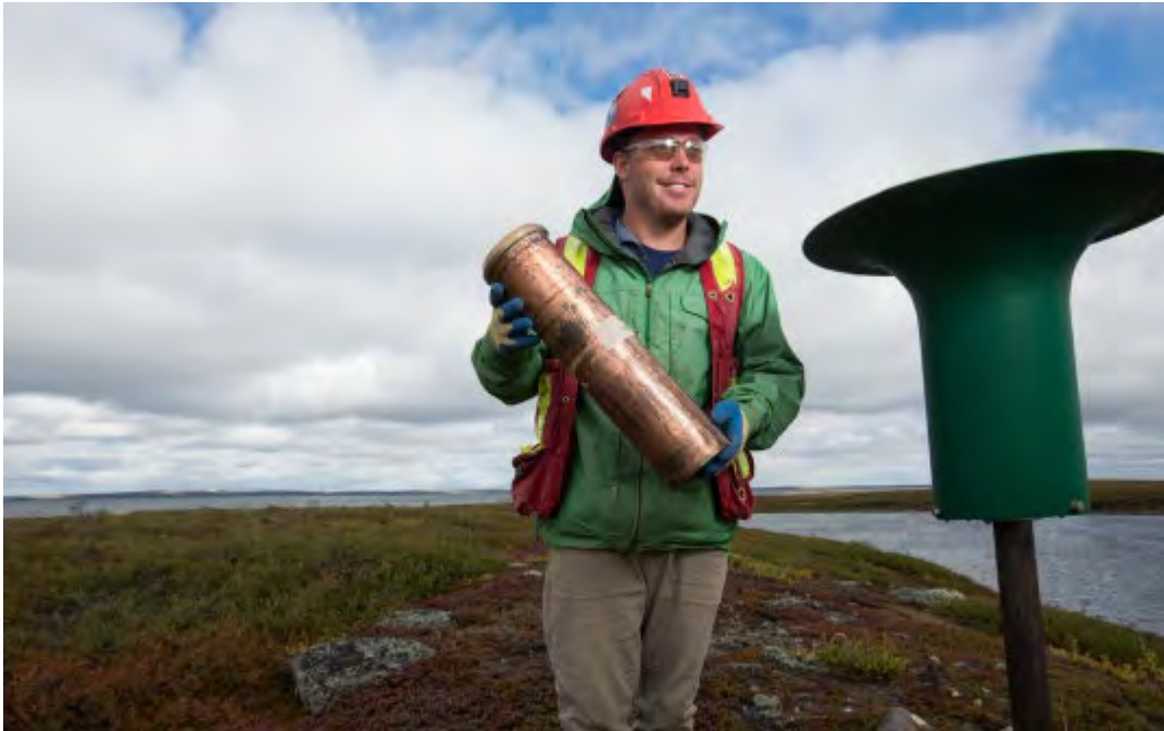
Photo 2-1 Dustfall gauge during sample collection. The dustfall gauge consisted of a hollow brass cylinder (centre) housed inside a Nipher snow gauge (right).
