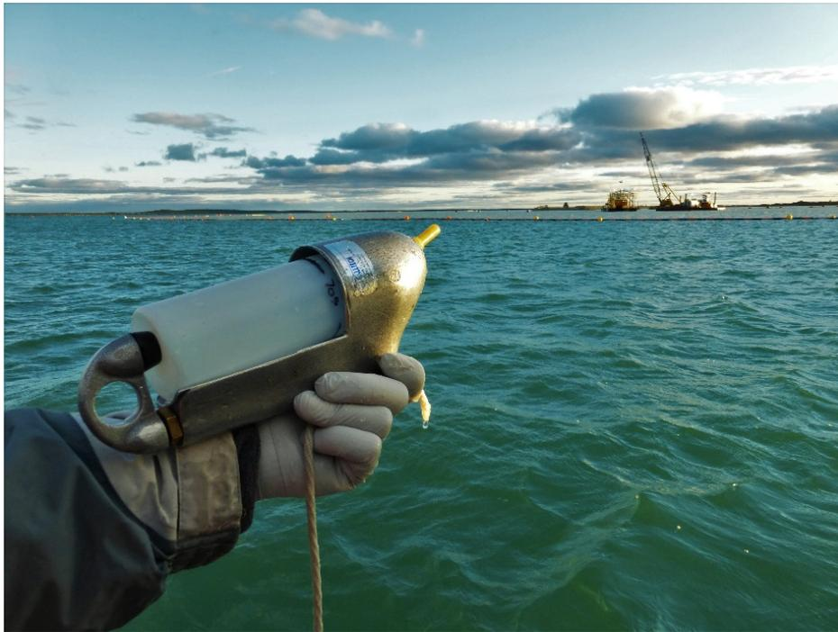
**Photo 4-1**      **Depth integrated sampler**
