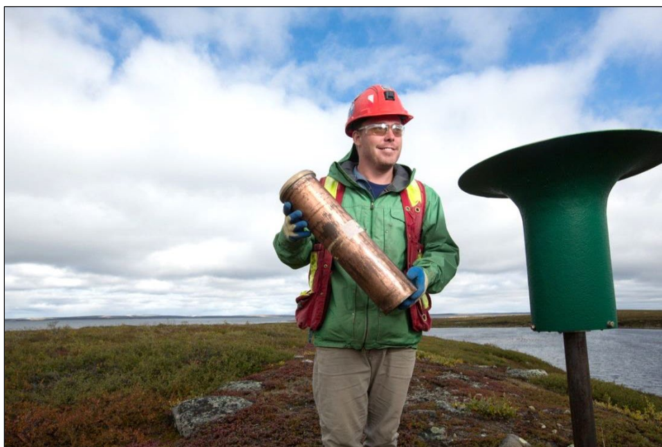
Photo 2.1-1: Dustfall gauge during sample collection. The dustfall gauge consisted of a hollow brass cylinder (centre) housed inside a Nipher snow gauge (right).
