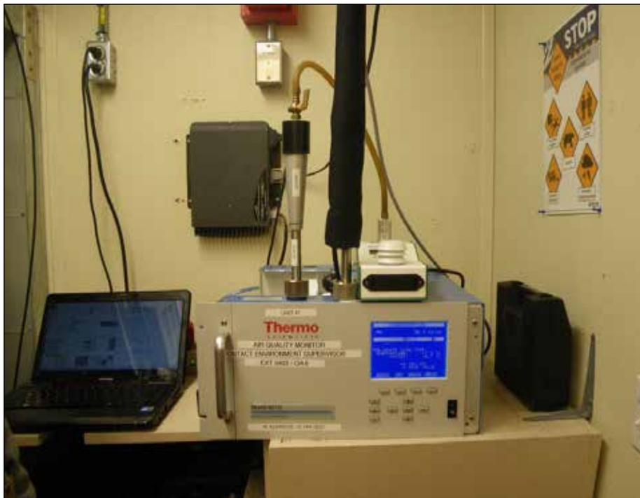
Plate 6. CB TSP Station calibrations and leak test.
