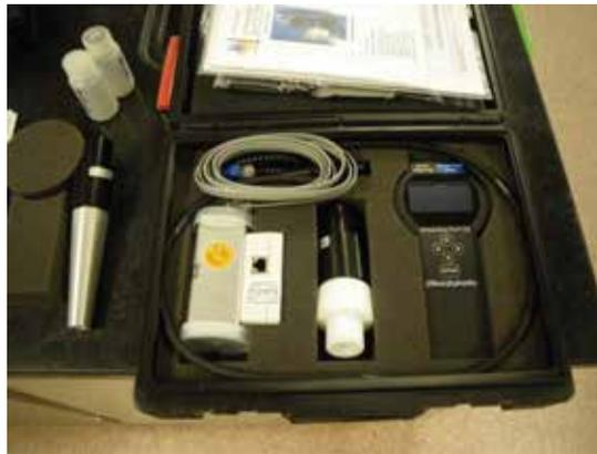
Plate 4. Streamline Pro and flow/leak check adapter on the left.
