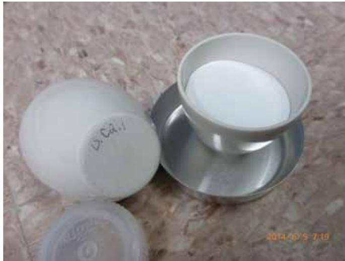
Photo 4: Ceramic Crucibles with filter
