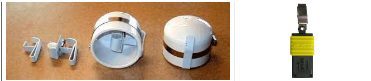
Figure 2: Example setup of passive samplers including personal badge
