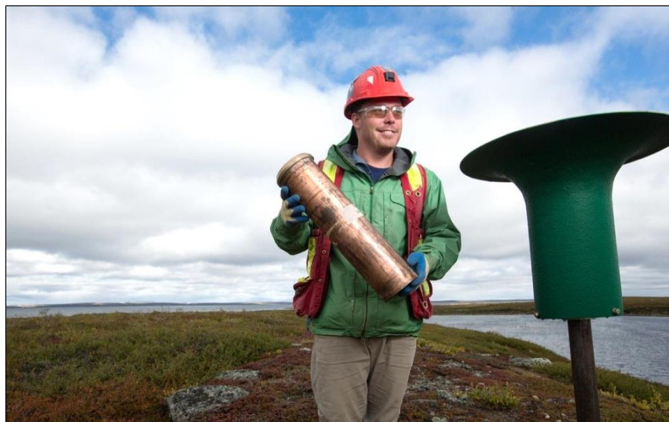
Photo 2.1-1: Dustfall gauge during sample collection. The dustfall gauge consisted of a hollow brass cylinder (centre) housed inside a Nipher snow gauge (right).
