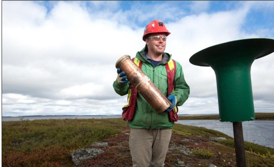
Photo 2.1-1: Dustfall gauge during sample collection. The dustfall gauge consisted of a hollow brass cylinder (centre) housed inside a Nipher snow gauge (right).
