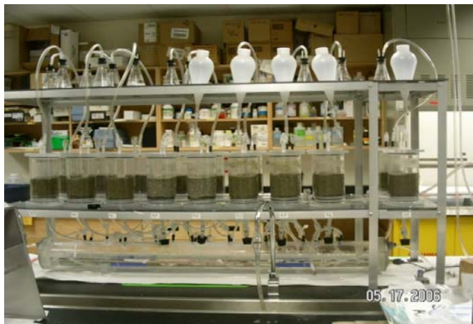
Figure 3-1. Room temperature humidity Cell Experiments
