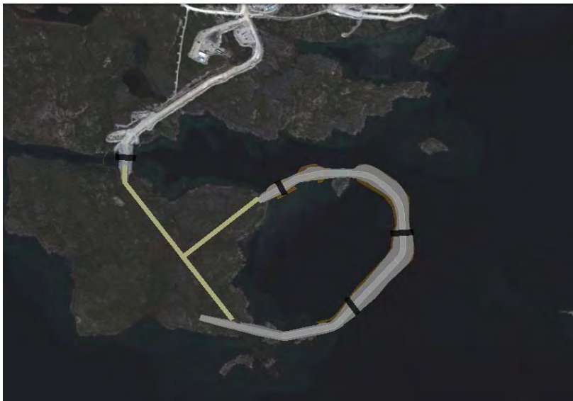
Figure 8-1. Closure concept for A21 pit and dike.
