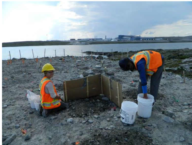
Photo 6. Seeding plots with native cultivars and applying Soil Lynx™ (erosion control material).
