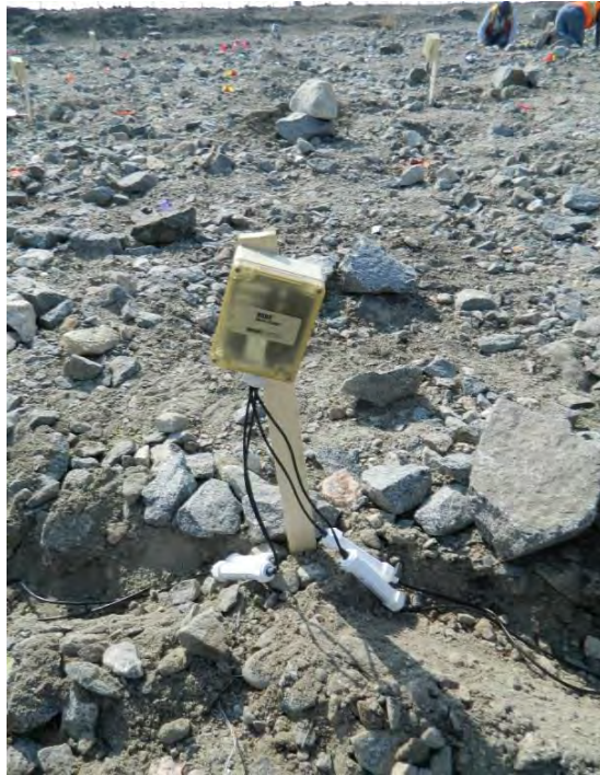
Photo 5. Installation of HOBO sensors to monitor soil water content and temperature.
