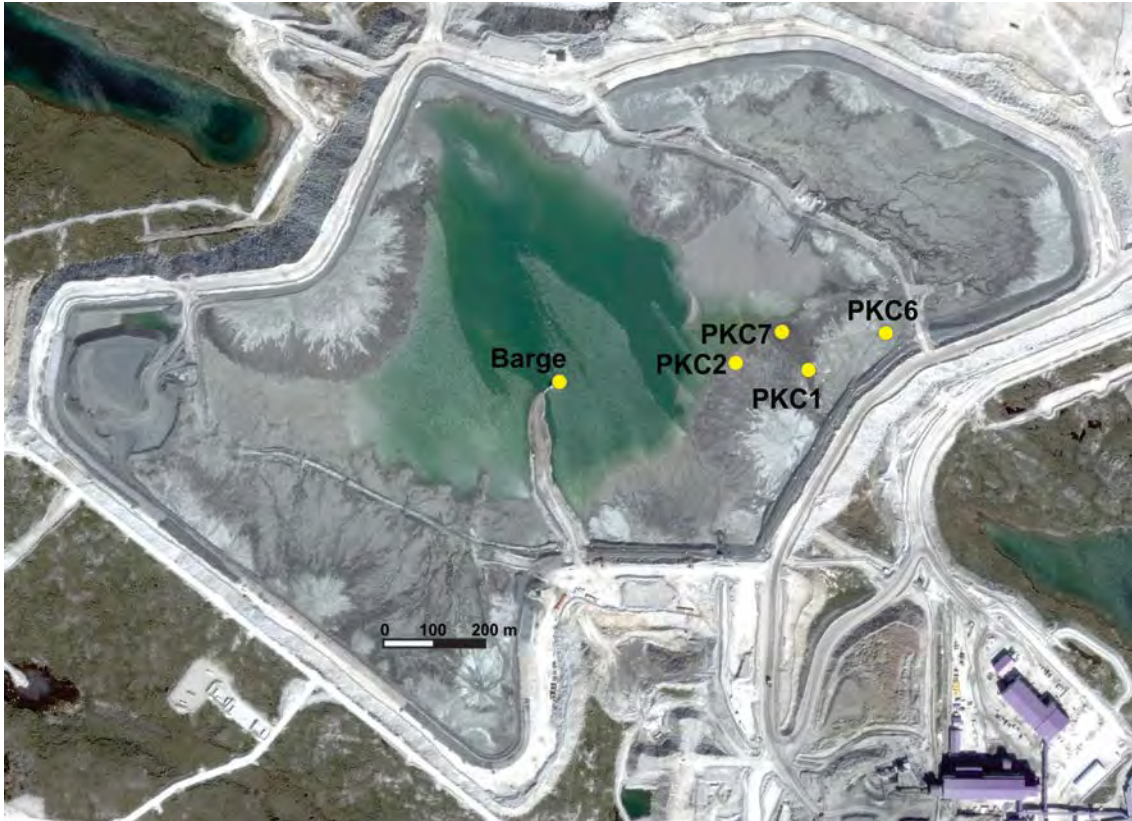
Figure 1: Aerial view of the PKC facility showing core collection and piezometer nest locations. The whitish-grey areas covering most of the brown-grey PK are secondary efflorescent minerals.
