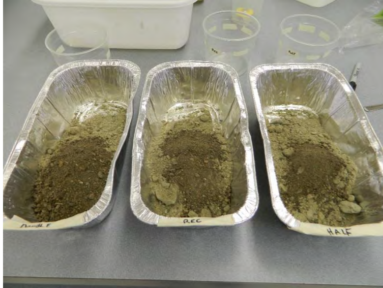
Photo 1. Mixing amendments and substrates (soil and till-sediment) at three rates for effects of water stress on vegetation growth and germination.
