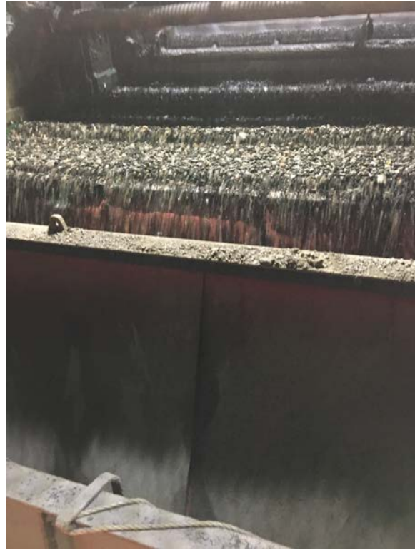
Multiple screens separate out crushed rock.
