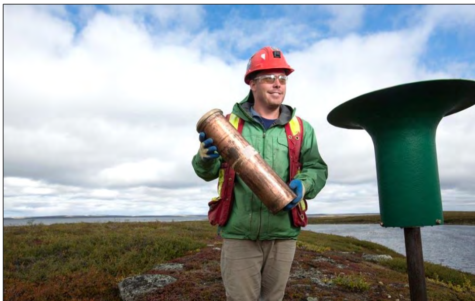
Photo 3.1-1: Dustfall gauge during sample collection. The dustfall gauge consisted of a hollow brass cylinder (centre) housed inside a Nipher snow gauge (right).
