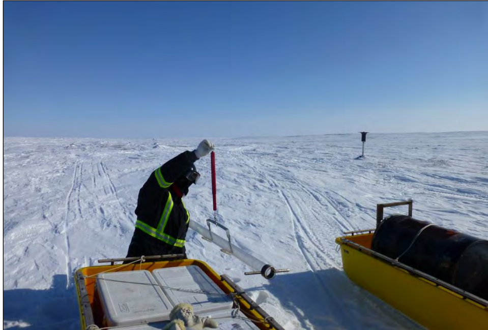
Photo 2.2-1: Snow core sample being weighed, with dustfall gauge in background.
