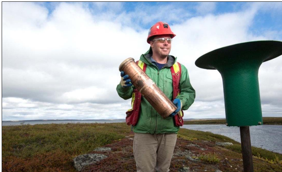
Plate 2.1-1. Dustfall gauge during sample collection. The dustfall gauge consisted of a hollow brass cylinder (centre) housed inside a Nipher snow gauge (right).
