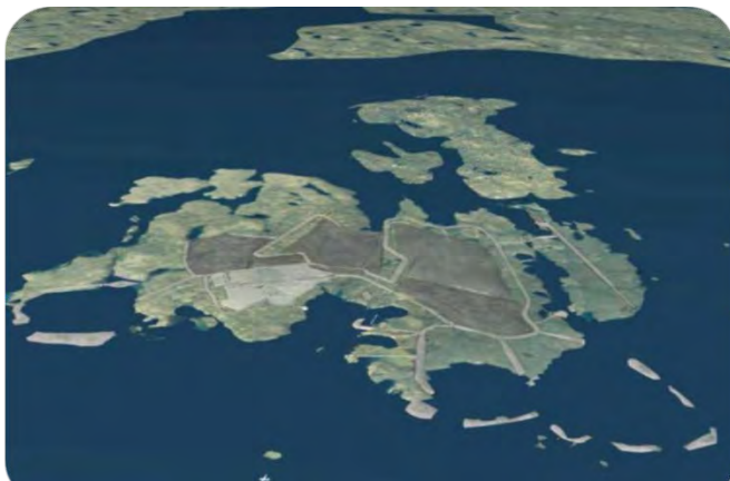
Figure 7: Depiction of currently approved closure plan with flooded pits, waste rock pile and PKC pond.
