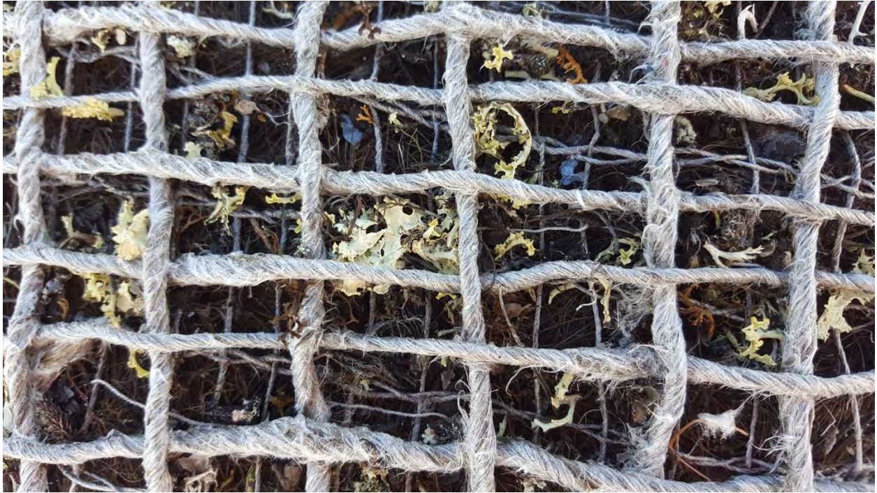
Photo 7. Good retention of lichen and soil biological crust with jute and erosion control blanket.
