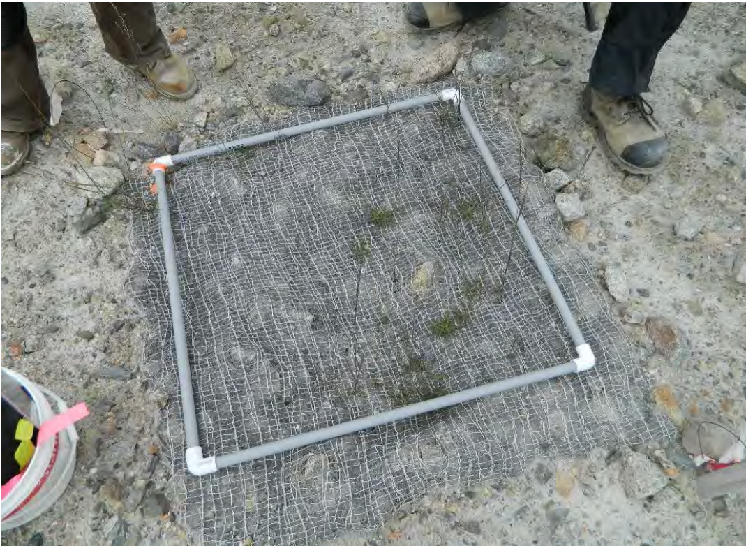
Photo 6. Plant growth on erosion control blankets.
