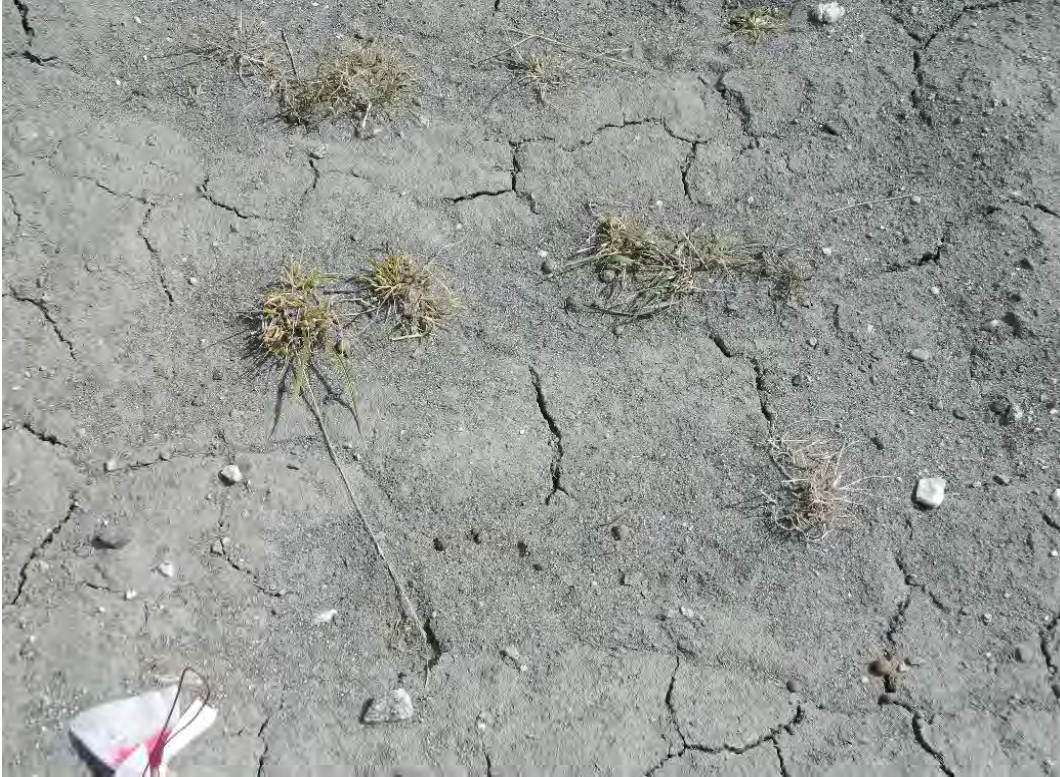
Photo 5. Furrows almost completely eroded in processed kimberlite.
