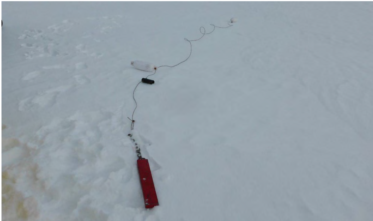
Photo 2-1 Temperature logger setup, Spring 2016.
