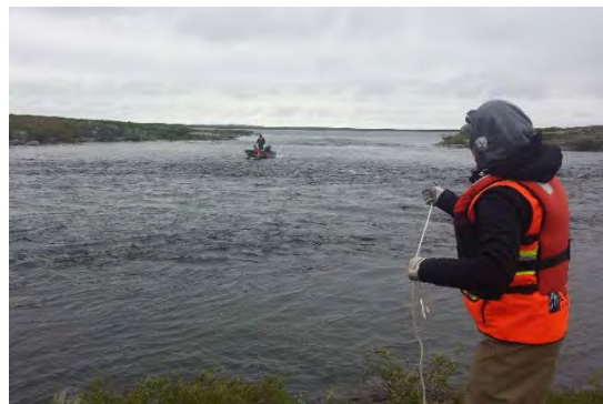
Photo 37: DDMI staff using boat to stretch antenna array across narrows
