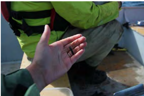
Photo 30: Example of HDX 23 mm PIT tag used
