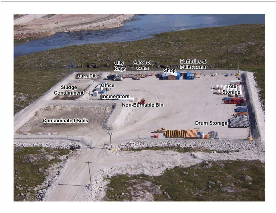
Figure 1: Waste Transfer Area Layout
