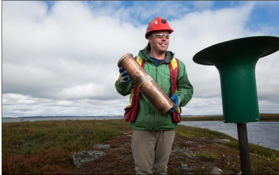
Plate 3.1-1. Dustfall gauge during sample collection. The dustfall gauge consisted of a hollow brass cylinder (centre) housed inside a Nipher snow gauge (right).
