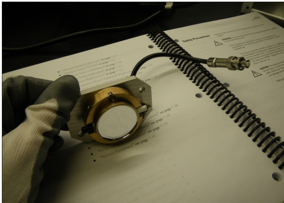
Plate 3. A154 Dike TSP Station replaced beta detector assembly.
