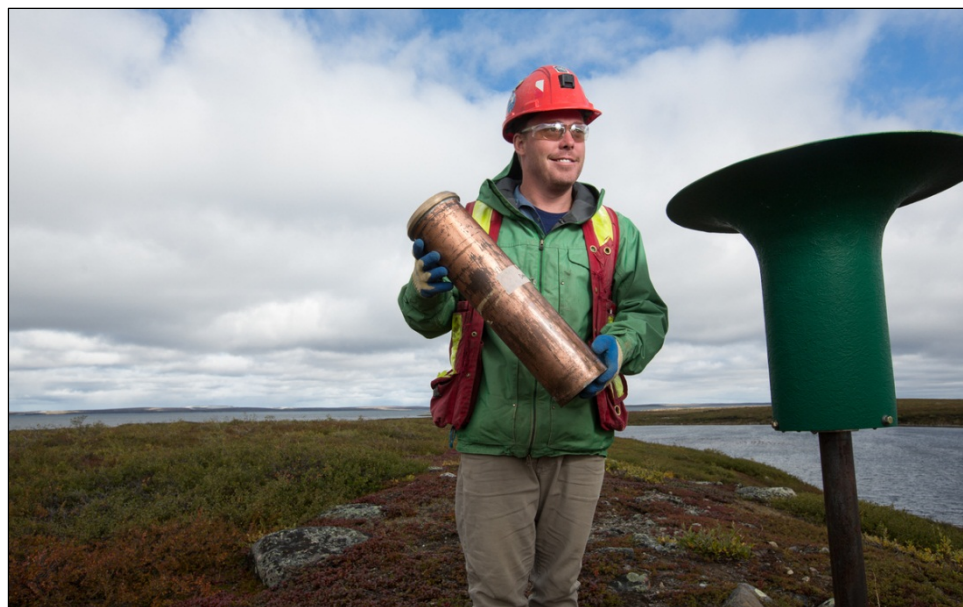
Plate 2.1-1. Dustfall gauge during sample collection. The dustfall gauge consisted of a hollow brass cylinder (centre) housed inside a Nipher snow gauge (right).
