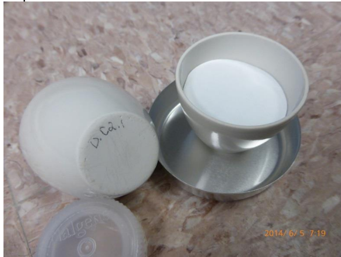
Photo 4: Ceramic Crucibles with filter
