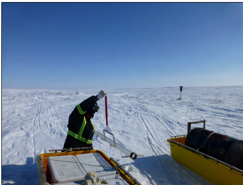
Plate 2.2-1. Snow core sample being weighed, with dustfall gauge in background.
