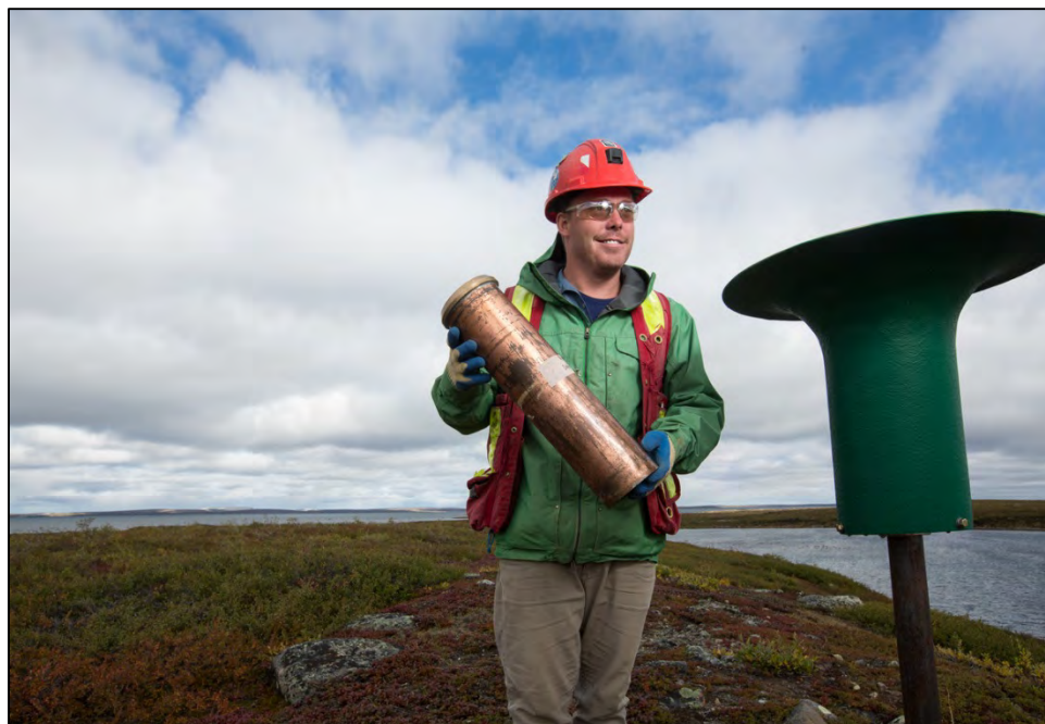
Plate 2.1-1. Dustfall gauge during sample collection. The dustfall gauge consists of a hollow brass cylinder (centre) housed inside a Nipher snow gauge (right).
