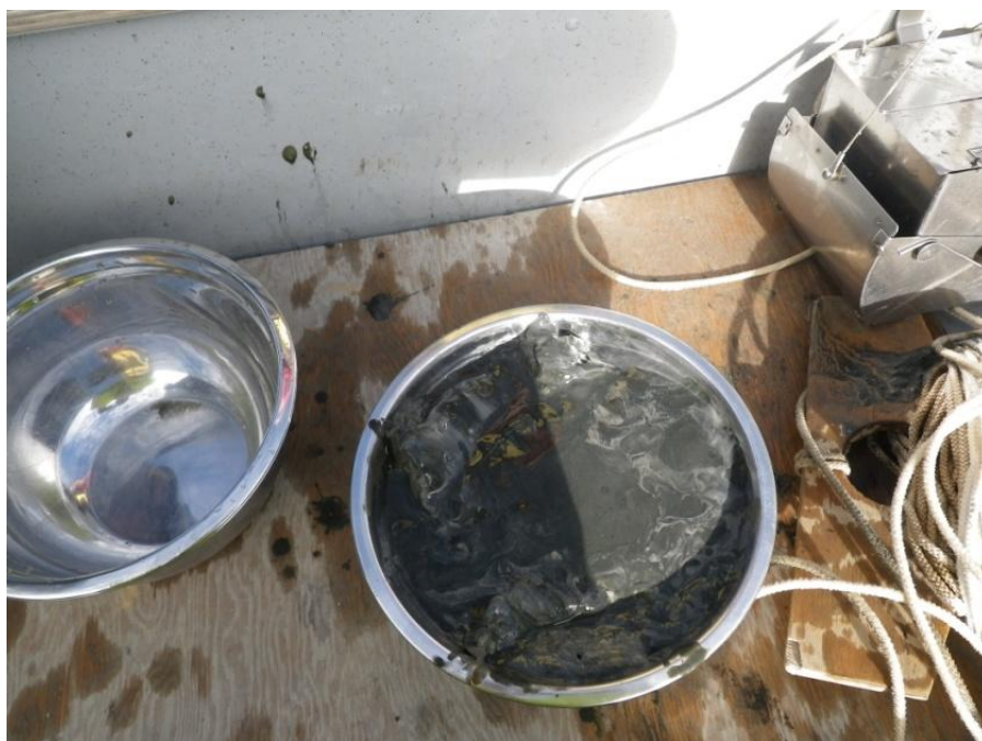
Figure 10: North Inlet reconnaissance: grab at transect location 4. Grab collected between Stations NI-1 and NI-2. Black/green layer (1 to 2 cm thick) overlying grey silt/clay; high water content in upper layer. UTM coordinates (UTM Zone 12): 533876 easting, 7153586 northing.
