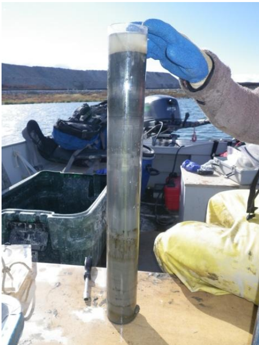
Figure 22: Station NI-2, third sediment core sample. Penetration depth: 56 cm. Approximately 7 cm of darker loose material at surface.
