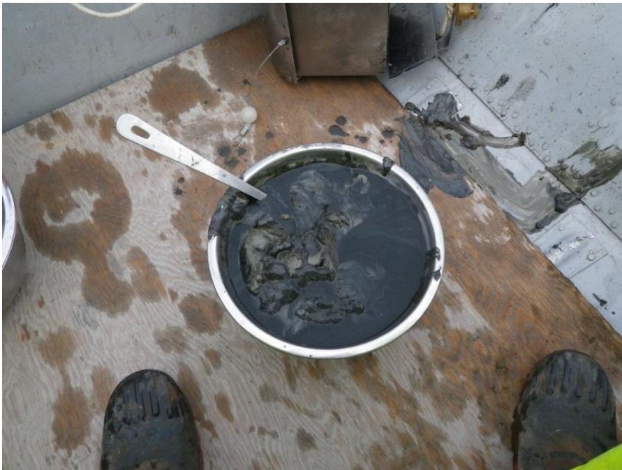
Figure 8: North Inlet reconnaissance: grab at transect location 2. Grab collected west of Station NI-1. Black/green slime layer approximately 2 cm thick overlying grey and brown silt and clay. UTM coordinates (UTM Zone 12): 533717 easting, 7153704 northing.
