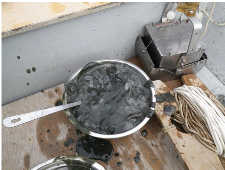
Figure 9: North Inlet reconnaissance: grab at transect location 3. Grab collected near Station NI-1. Black/green layer (1 to 2 cm thick) overlying grey silt/clay; high water content in upper layer. UTM coordinates (UTM Zone 12): 533806 easting, 7153649 northing.
