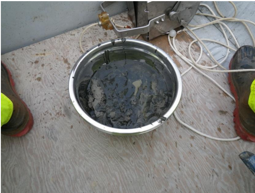
Figure 7: North Inlet reconnaissance: grab at transect location 1. Grab collected west of Station NI-1. Green/black algae and slime layer overlying very fine silt and clay. UTM coordinates (UTM Zone 12): 533617 easting, 7153717 northing.
