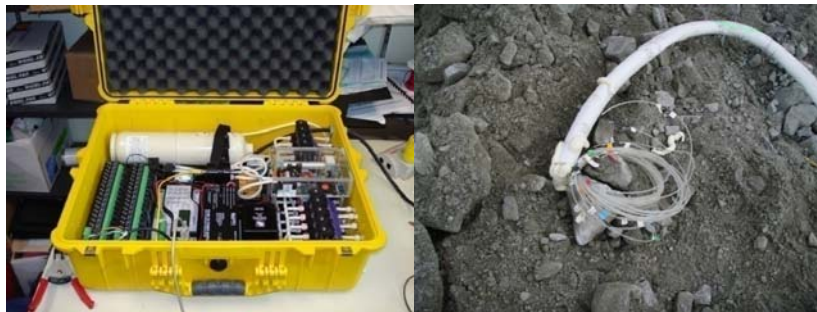
Figure 2-2. Portable 22 port O 2 /CO 2 sampler and gas sample tubing bundle.
